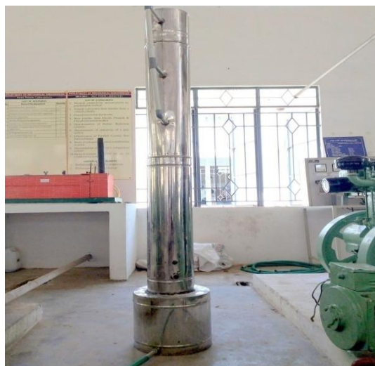
Fig.3 Dual type scrubber setup
