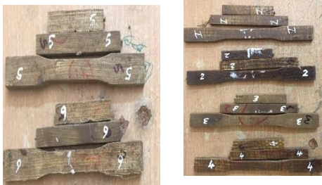
Fig 1: E-GF( 25%)+Resin (75%)+ vajram (85%)+ Epoxy(15%) plate
