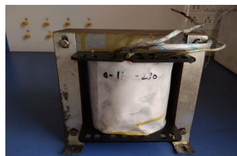
Figure 1: Photograph of 2 KVA single phase shell type Transformer
