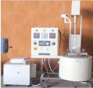
Fig.1. Stir casting setup
