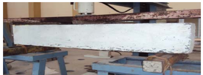
Fig 8 Experimental Setup For Flexural Behaviour of Concrete
