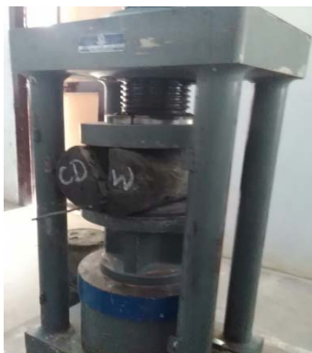
Fig.6.2 Tensile test on geopolymer concrete
