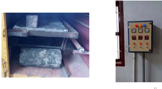
Fig.6.1 Curing of geopolymer concrete
