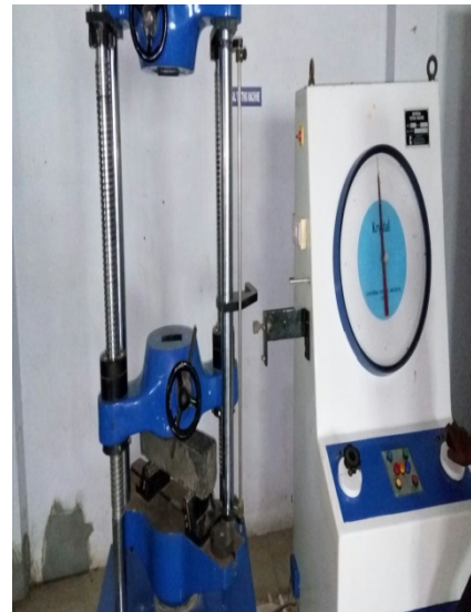
Fig.6.3 Flexural test on geopolymer concrete
