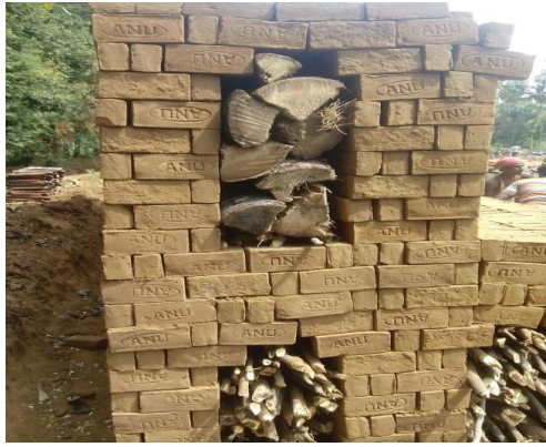
Fig 4 Burning of Bricks
