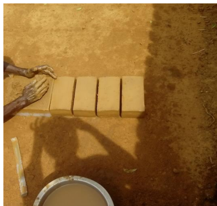
Fig 2 Moulding of Bricks
