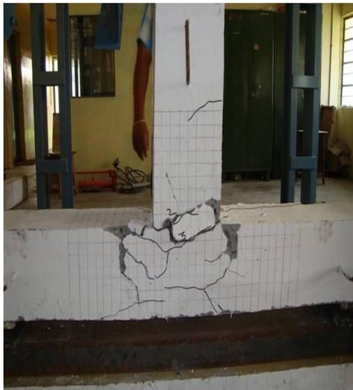
**Figure 7 Typical View of Failed Control Specimen**
