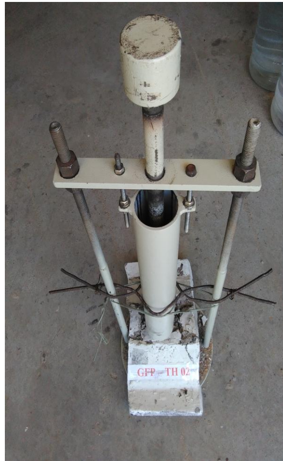
Figure 2. impact machine set-up
