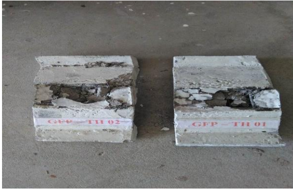
Figure 7. Geopolymer Ferrocement Trough Panels at failure
