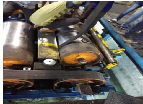
Fig 3. Workers fixing the damaged rollers
