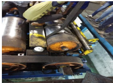
Fig 3. Workers fixing the damaged rollers
