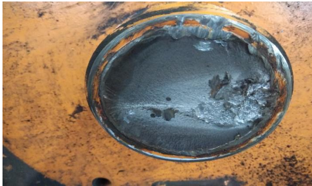
Fig.4. Failure due to brittle effect
