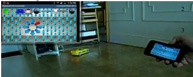
Figure 8: The robot moves in the direction of the movement of the users hand: forward –right.
