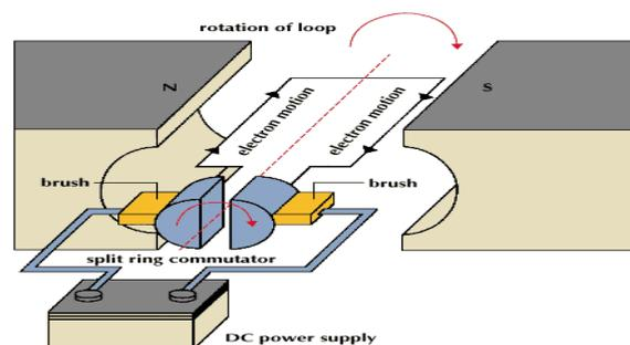
**Fig 9: Operation of a DC Motor**
