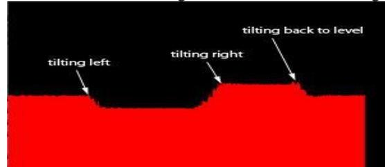
This graph shows the Y axis. The accelerometer starts level, and then is tilted forward, then back, then level again:
