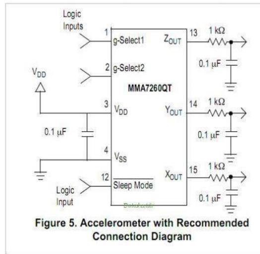
The pins of the accelerometer are as follows:
