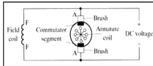
**Fig 8: Simple diagram of DC motor**
