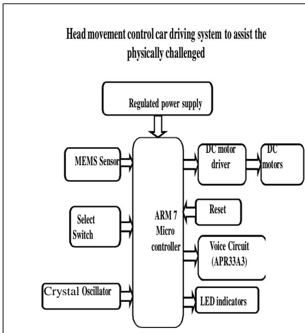
**FIG 1: Block diagram of HEAD MOVEMENT CONTROL CAR DRIVING SYSTEM TO ASSIST THE PHYSICALLY CHALLENGED**
