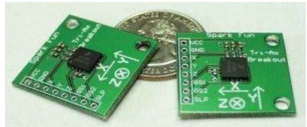
**Fig 2 MEMS sensor MMA7260Q**
