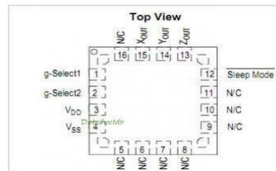
**Fig3 MEMS PIN DIAGRAM**
