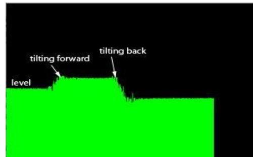
This graph shows the Z axis. The accelerometer is kept level, but raised up in a quick motion, then lowered quickly. Moving up produces a sudden increase in force (and voltage) followed by a sudden decrease when the movement's stopped, then finally the voltage levels out again. Moving down has the opposite effect.
