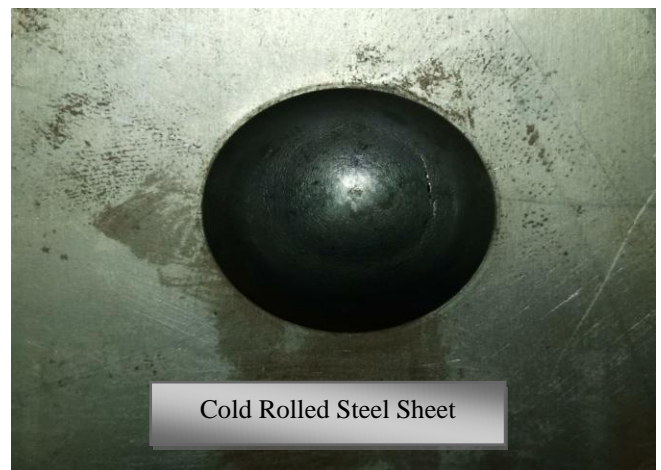
Fig.8 Cold Rolled Steel Sheet after deformation
