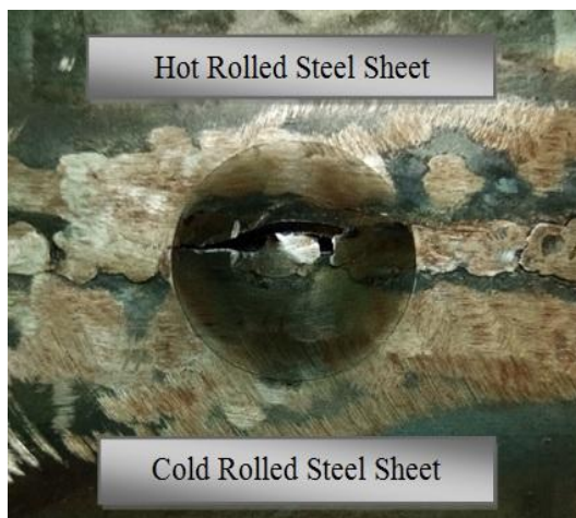
Fig.10 Gas welded sheet (both hot rolled and cold rolled) after deformation
