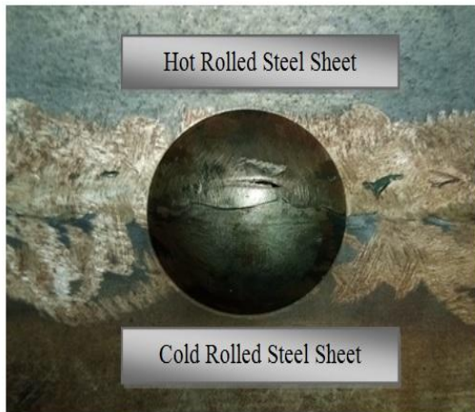
Fig.9 TIG welded sheet (both hot rolled and cold rolled) after deformation
