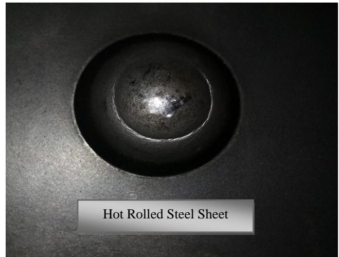
Fig.7 Hot Rolled Steel Sheet after deformation
