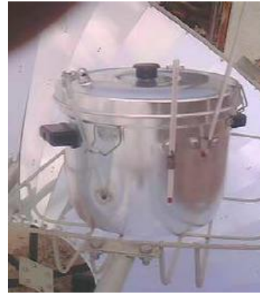
Fig: 2 Thermometers used for Temperature Measurement
