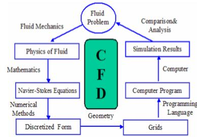
**Fig 6.1 Process of CFD**
