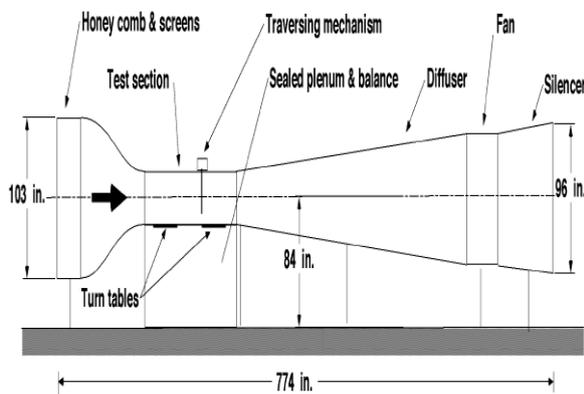
**Fig.1.2.1 Model prepared for the wing tunnel testing**
