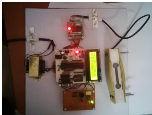
Figure 2.4 Setup for Predetermination of Fatigue and Fracture in Glass Fibre Reinforced Composite Laminate
