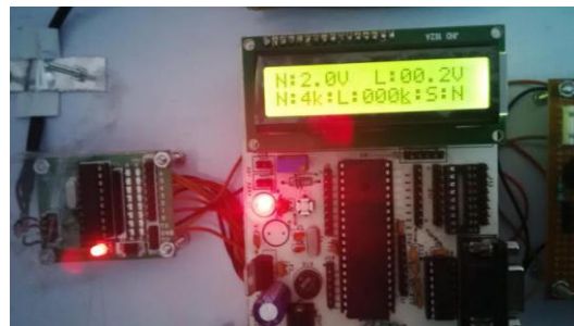
Figure 2.7 As the load reaches 4kgs. Red light indicator glows
