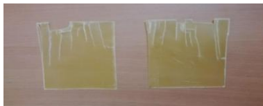
Figure 2.2 Fracture in glass fibre reinforced composite laminate
