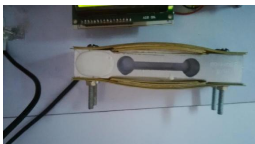
Figure 2.5 Glass fibre reinforced composite laminate attached to a load cell
