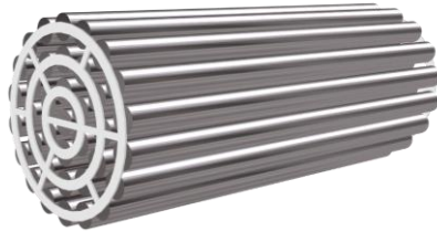
Fig 2: Modelled Fuel bundle in CATIA-V5
