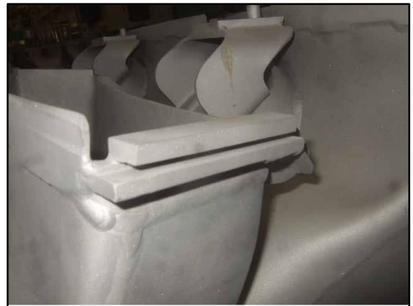
Wear in Transition piece Side Seal
