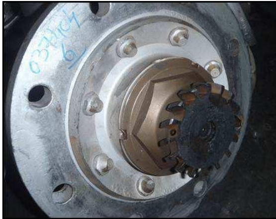
Gas Turbine Fuel Nozzle (plugged)
