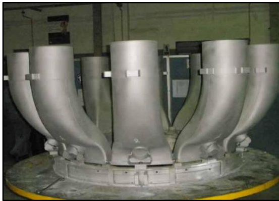
Gas Turbine transition piece assembly
