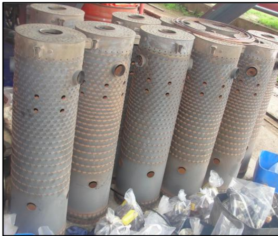
Gas Turbine combustion liners
