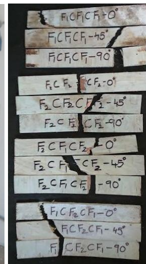
Fig.6: Specimens after tensile test
