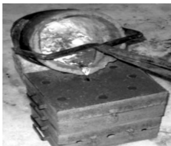
Fig 3: pouring the liquid metal into the casting
