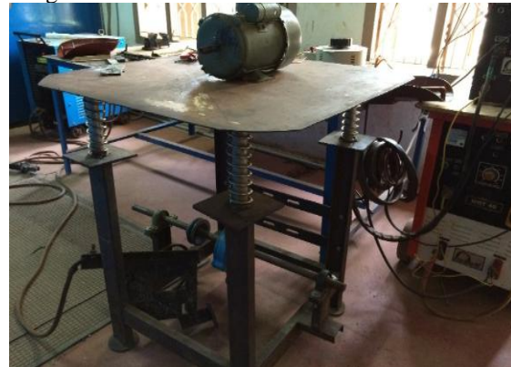
Fig. 3 Vibratory table setup
